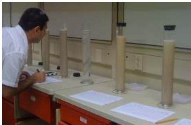
Figure 3.31. Typical hydrometer test reading recorded.
