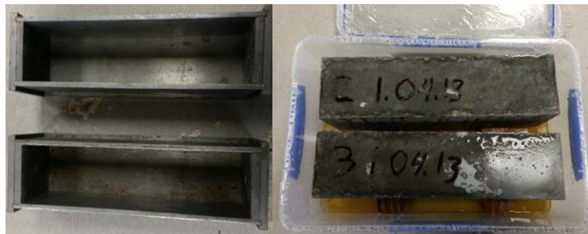
Fig. 3.2-3 Typical CPT prism molds (left), and storage containers (right).
