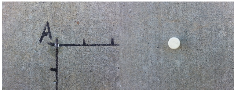
Fig. 3.3-2 Typical gage stud (left) and humidity port with cap (right).
