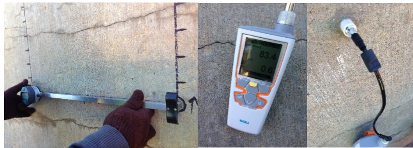
Fig. 3.3-3 DEMEC gage during length-change measurement (left), portable humidity indicator (center), and humidity probe inserted into a humidity port (right).
