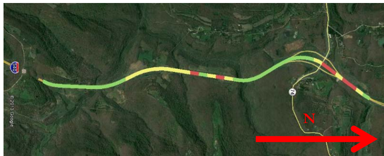
Fig. 4.1 Median barrier deterioration level along Interstate 49. Figure produced in Google Earth.
