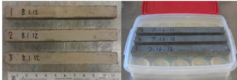
Fig. 3.2-2 Mortar-bars (left) and mortar-bar in storage container (right).
