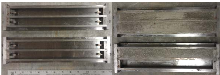
Fig. 3.2-1 Mortar-Bar mold with gage studs (left) and mortar-bar mold with three mortar-bars (right).
