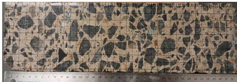
Fig. 3.2-4 Typical prepared DRI sample with grid.
