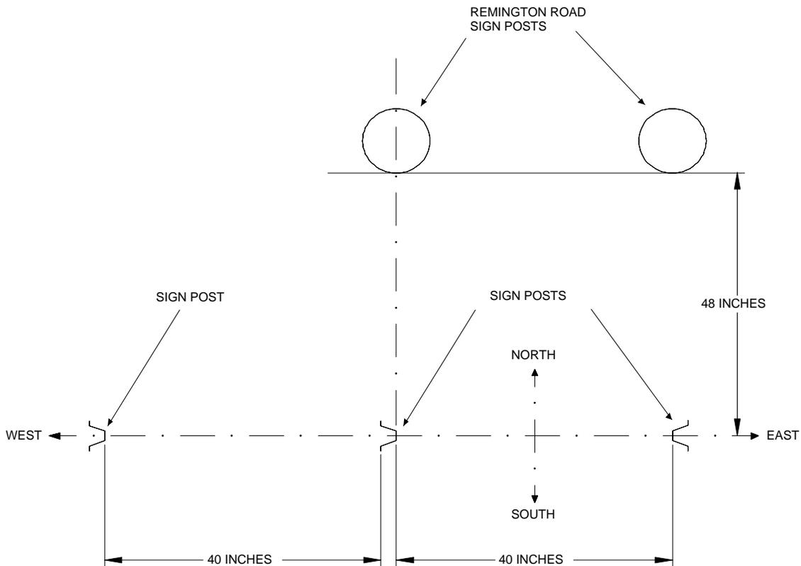
Fig.21 - Top View – Post Placement for Solar Panels & Control Boxes
