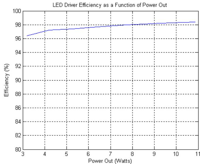
Fig.31 LED Driver Efficiency
