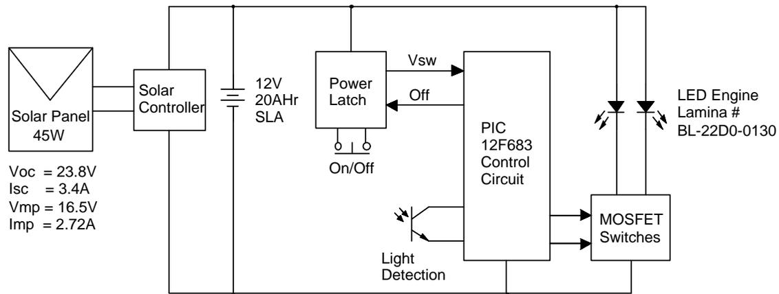
Fig.4 LED System Block Diagram
