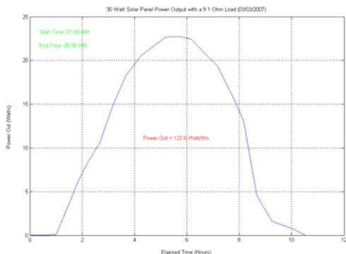
Fig.3a - Resistive Load
