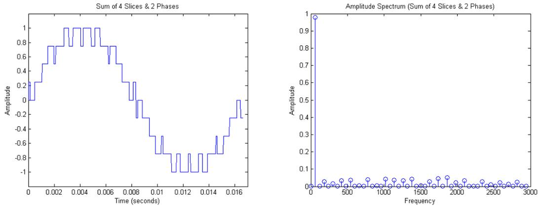
Fig.13 Simulated S-PWM of 4 Sections & 2 Phases (THD = 14.53%)
