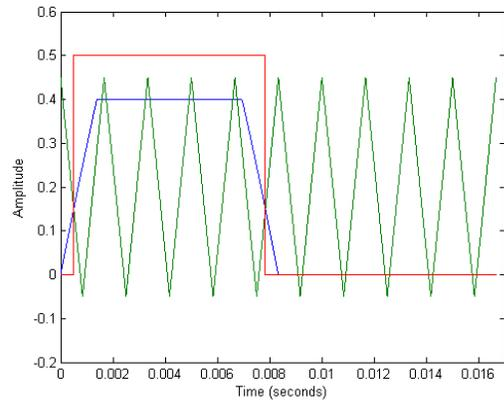
Fig.12c Sectionalized PWM of Section 3 ( $0^\circ$  &  $180^\circ$  Carrier)
