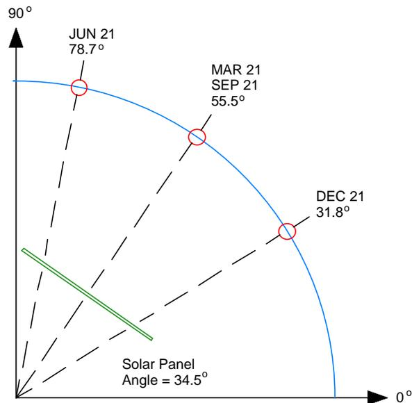
Fig.23 Solar Panel Orientation
