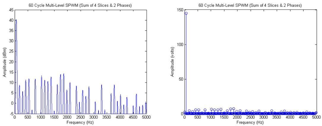
Fig.20 Frequency Spectra of Experimental S-PWM (THD = 14.54%)
