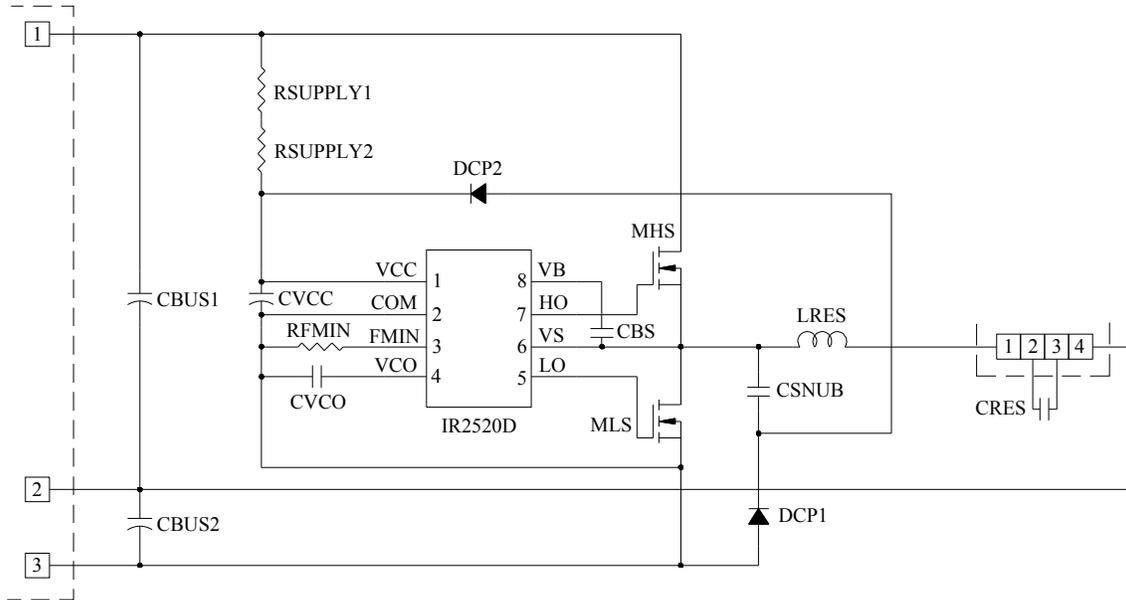
Fig. 45 Electronic Ballast
