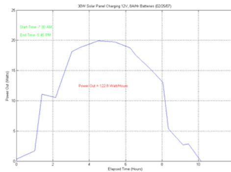
Fig.3b – Charging 12V Battery
