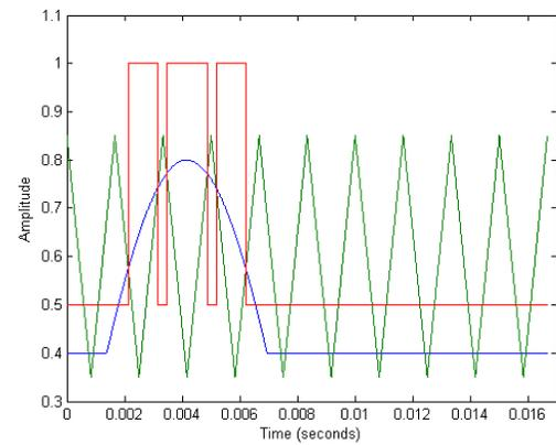
Fig.12d Sectionalized PWM of Section 4 ( $0^\circ$  &  $180^\circ$  Carrier)
