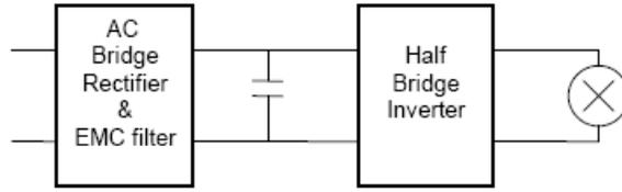
Fig. 39 Block Diagram of CFL Ballast
