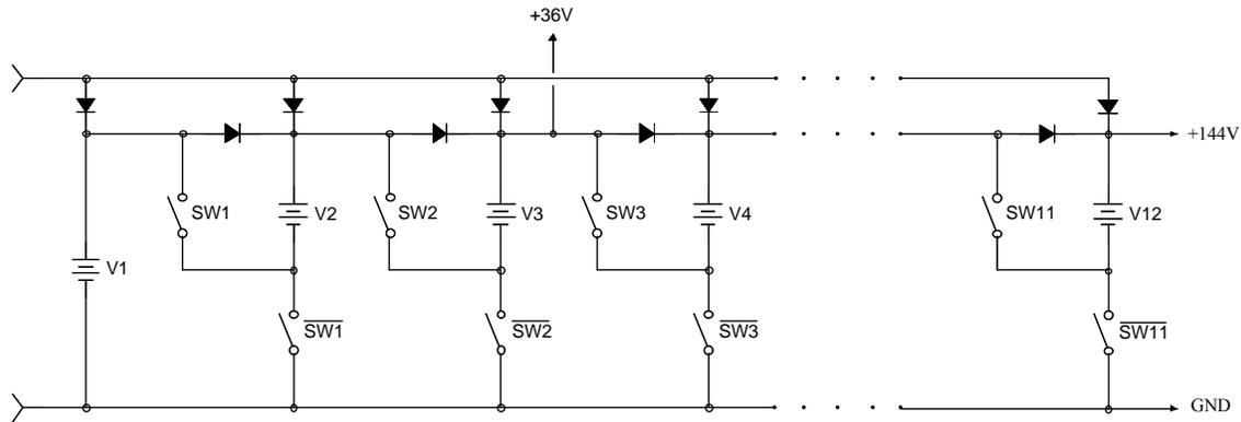
Fig.15 Battery Bank Switching Diagram
