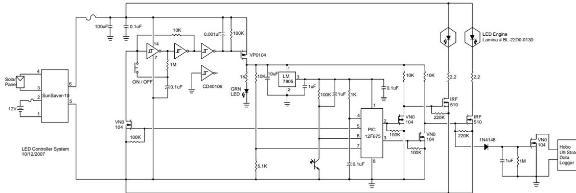
Fig.5 LED Driver Schematic
