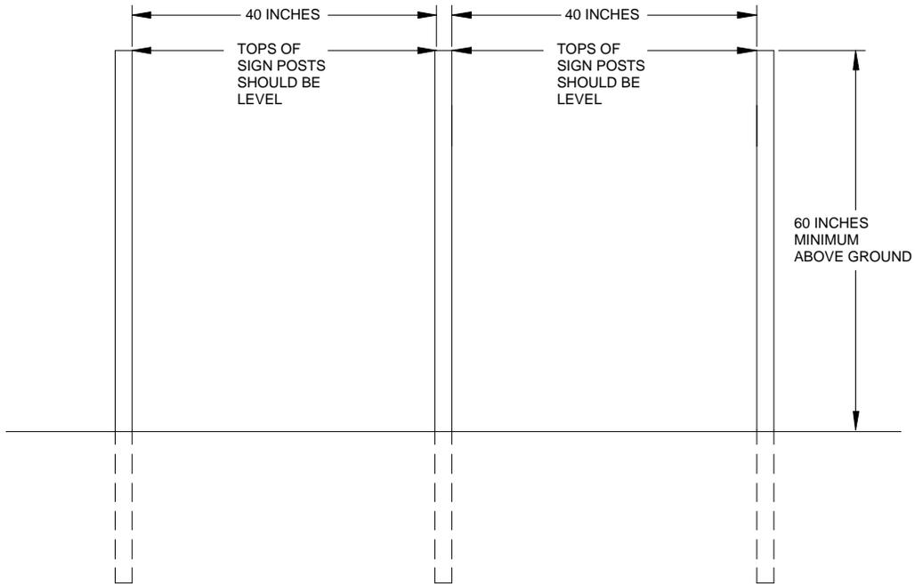
Fig.22 – Front View – Post Placement for Solar Panels & Control Boxes
