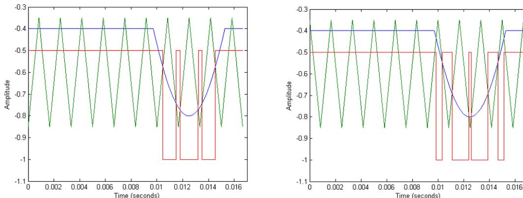
Fig.12a Sectionalized PWM of Section 1 ( $0^\circ$  &  $180^\circ$  Carrier)
