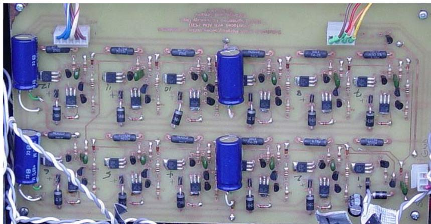
Fig. 16 Battery Bank PC Board
