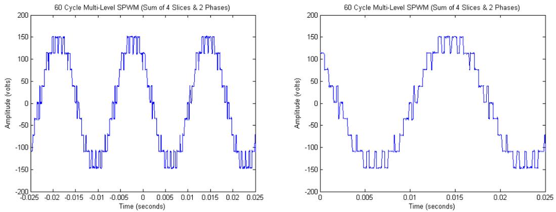
Fig.19 Experimental S-PWM – Captured on DOS & Plotted in MatLab
