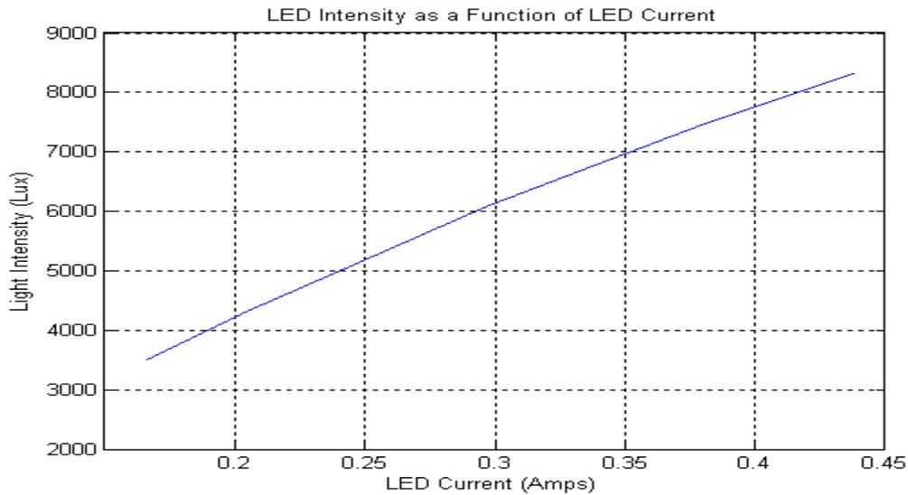
Fig.1 Plot – LED Intensity vs. LED Current
