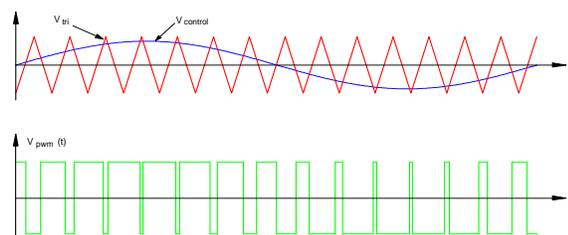
Fig.8b Sine Triangle PWM (SPWM)
