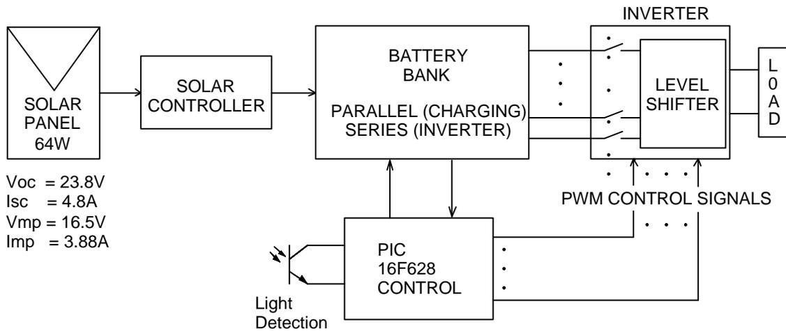
Fig.14 CFL System (DC/AC Inverter) Block Diagram
