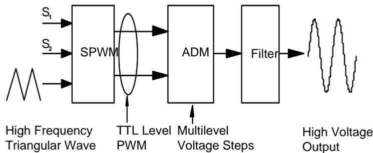
Fig.11 Multilevel SPWM Scheme
