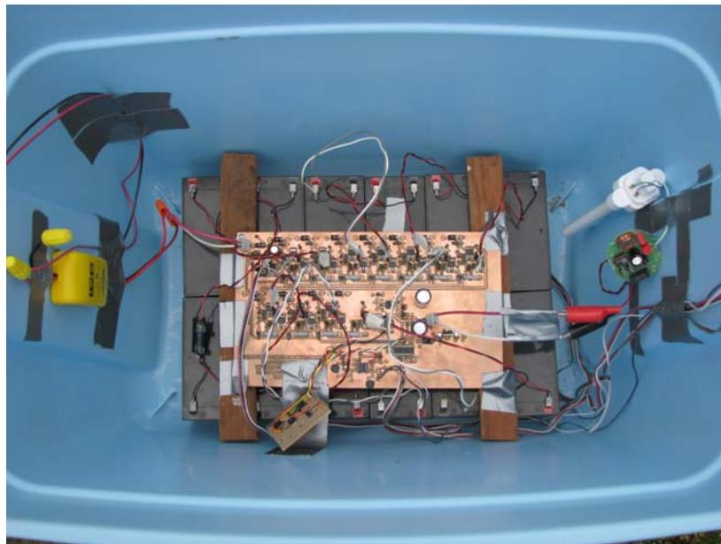
Fig. 46 26W CFL PCB & Light System Setup
