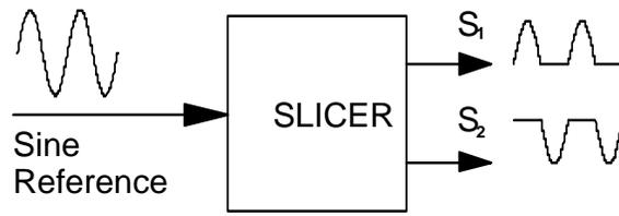
Fig.10 Slicing Reference Signal into Two Halves
