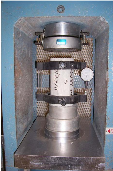
**Figure 3.11 Modulus of Elasticity Apparatus**
