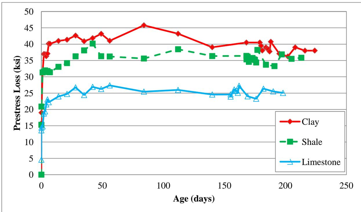
**Figure 4.4 Measured Losses: Comparison of Different Aggregates**
