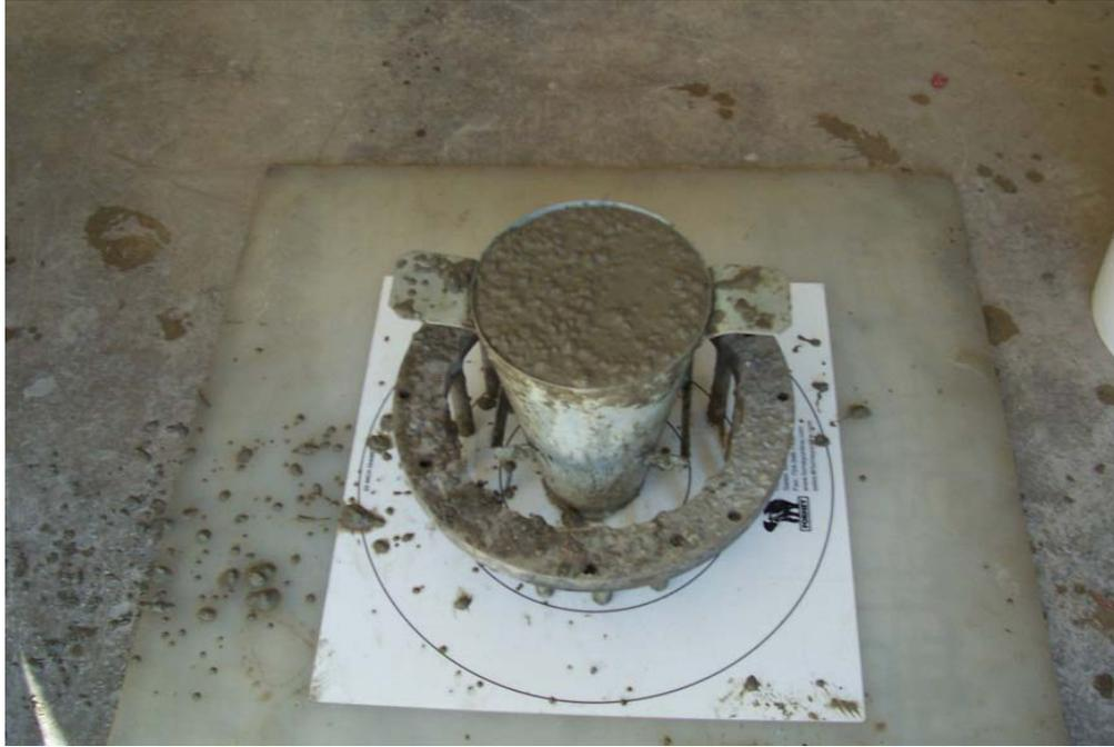
**Figure 3.9 J-Ring Test Part 1: Fill the Cone**
