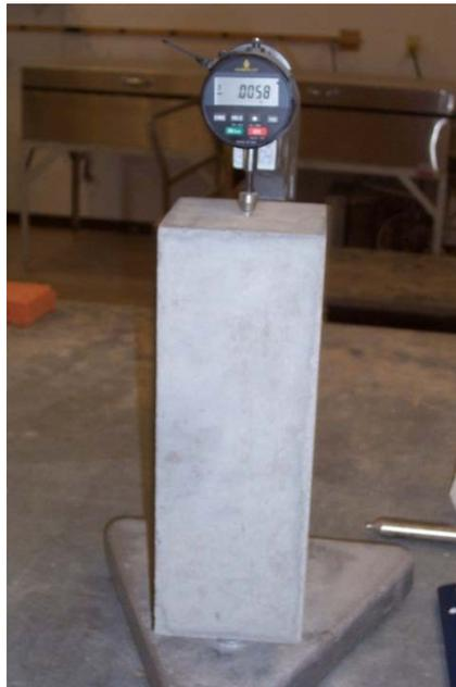
**Figure 3.12 Prism Resting in Shrinkage Apparatus**
