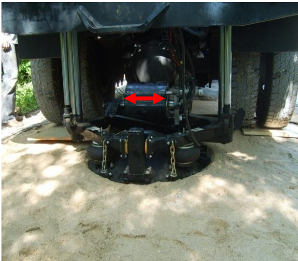
Figure 3.20: Shear loading configuration.
