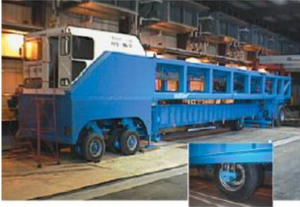
Figure 2.1: Heavy Vehicle Simulator (Perkins et al. 2005).
