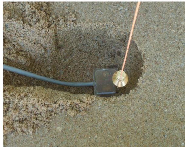
Figure 3.15: Geophone package placement three inches deep in sand lift.
