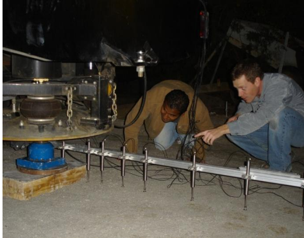
Figure 4.13: Monitoring the deformation of the test section during loading.
