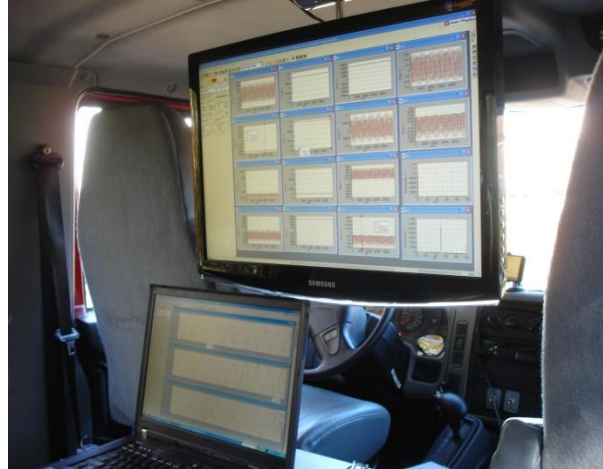
Figure 4.14: Monitoring the LVDTs output signals during loading.
