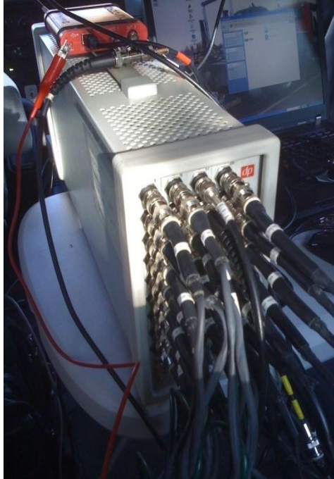
Figure 3.25: Data Acquisition System.
