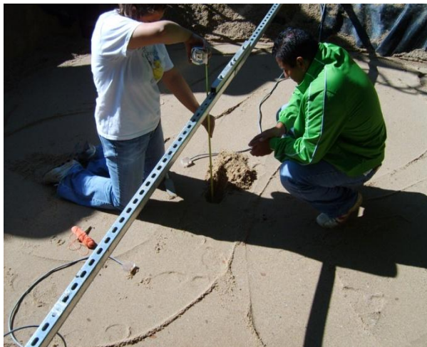
Figure 3.14: Geophone package placement measurements.
