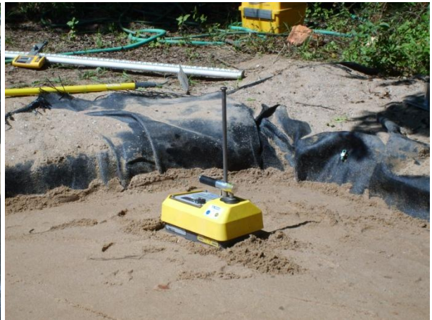
Figure 3.12: Nuclear density gauge reading.
