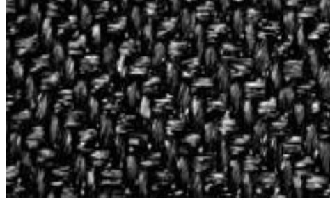
Figure 3.3: Geotextile used in this project (Mirafi® HP570) ( www.tencate.com ).
