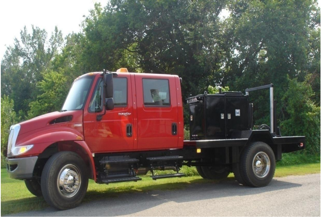
Figure 3.19: University of Arkansas' Vibroseis truck.
