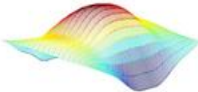
Mode 10: Deck First Bending Mode (34.7Hz)
