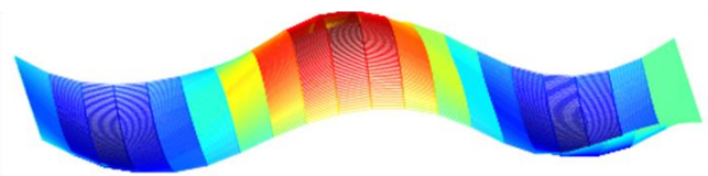
Mode 9: Third Bending Mode (40.4 Hz)
