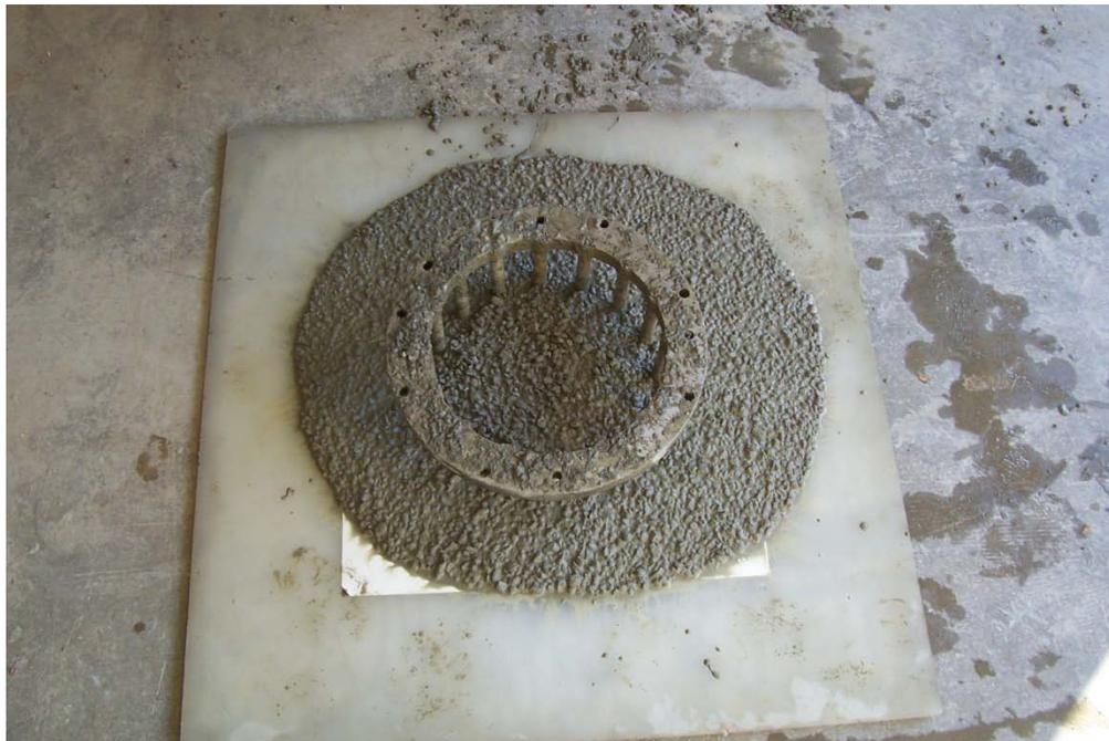
**Figure 3.10 J-Ring Test Part 2: Measure the Flow**
