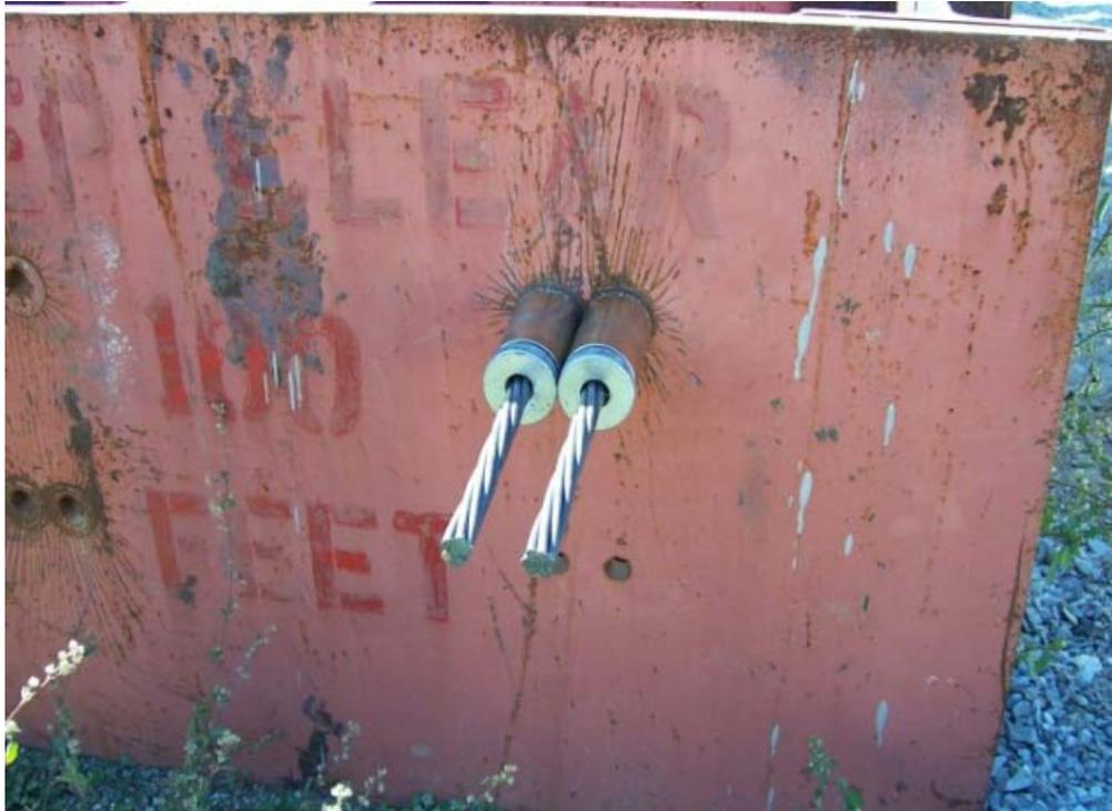
**Figure 3.7 Anchorage Chucks**
