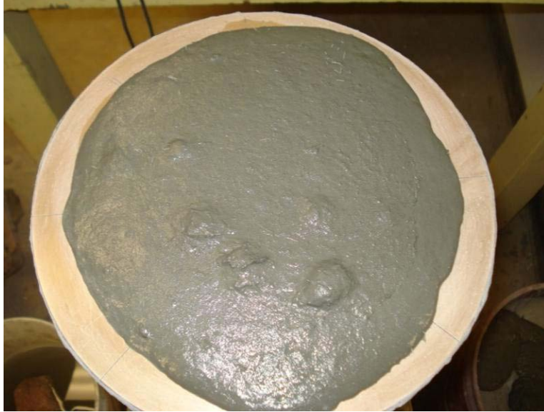
Figure 4.19 Unmixed Portions of Premix Material Contained on Flow Table.
