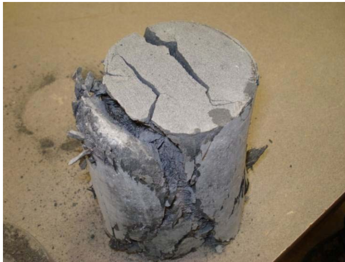
Figure 2.1 Typical UHPC Cylinder Failure.
