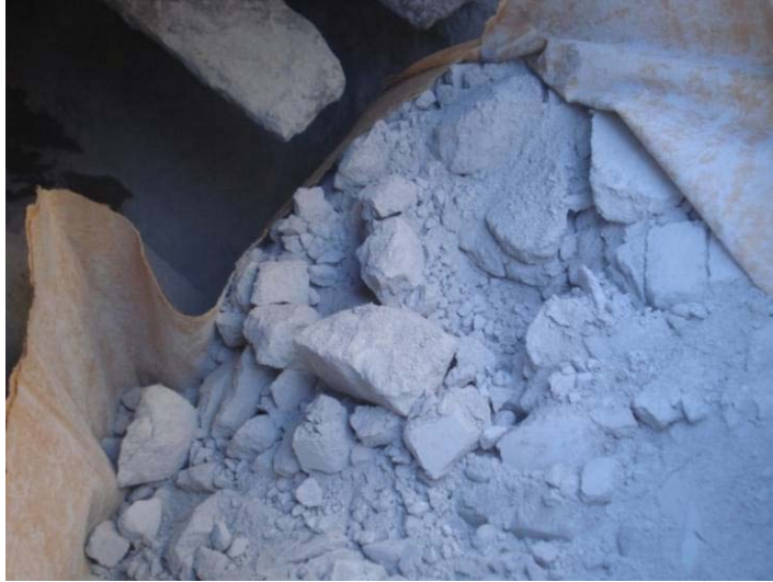
Figure 3.4 Evidence of Dry Premix Agglomerations.
